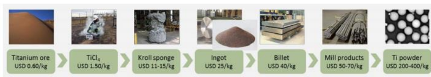
Titanium metal production flowsheet and value accretion at each production stage (Kroll process)
