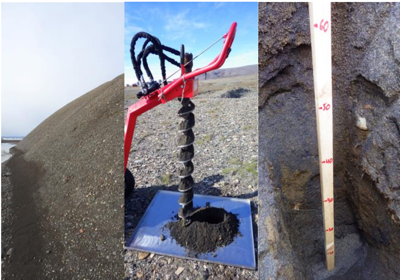
Figure 5 - (LHS) Auger sample from raised beach – the black material is ilmenite rich sediment; (RHS) Initial trenching demonstrating ilmenite depositional modes; The black banding is virtually pure ilmenite
